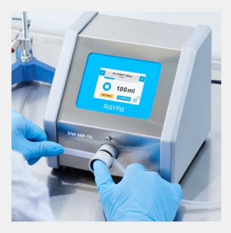
**2.** Place the dispensing line inside the pinch solenoid valve of the external dosing station.
