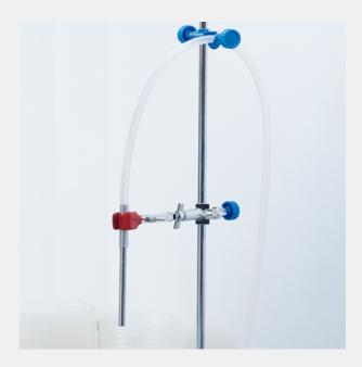
**3.** Place the clamps on the vertical stand at the desired height, ensuring the line's metal part is fastened by the lower clamp.
